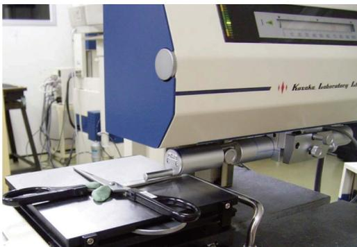
Fig. 1 Measurement of the primary profile
